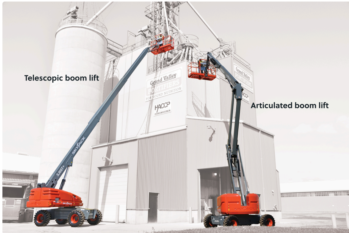
Telescopic boom on the left and Articulating boom on the right.
